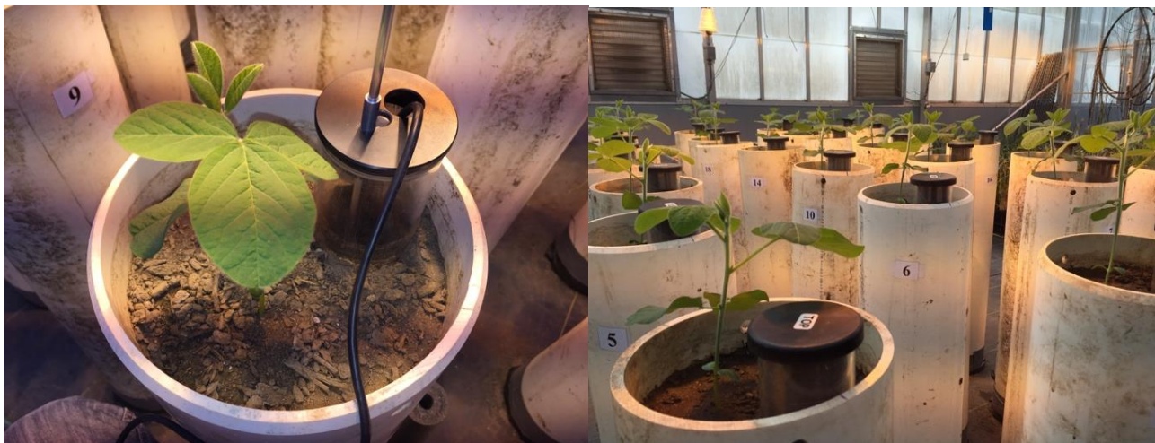
Figure 1. Transparent acrylic minirhizotron tube placed vertically inside each growing column to facilitate root imaging. Manhattan, Kansas, United States.
